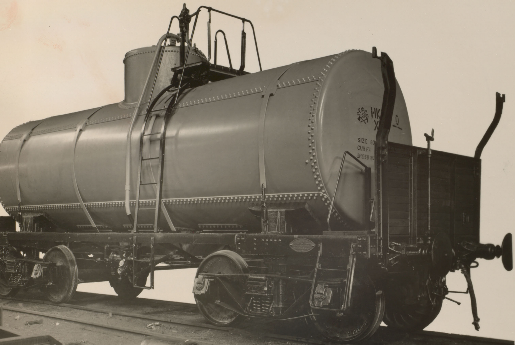
C1394. MONTREAL WORKS - CC & FG - OCT 1921 - 8000 WINE GALL TANK CAR FOR RUSSIAN SOVIET GOVERNMENT
