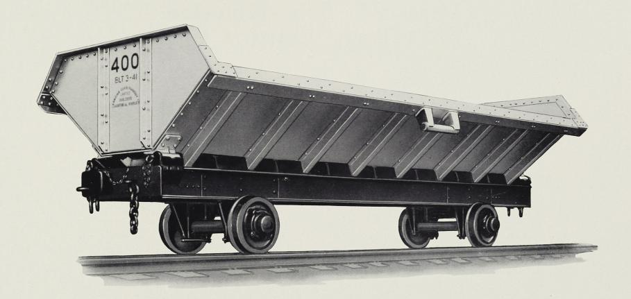
11 cu. yd. Four-Wheeled Side-Dump Quarry Car Shipped to British Guiana
