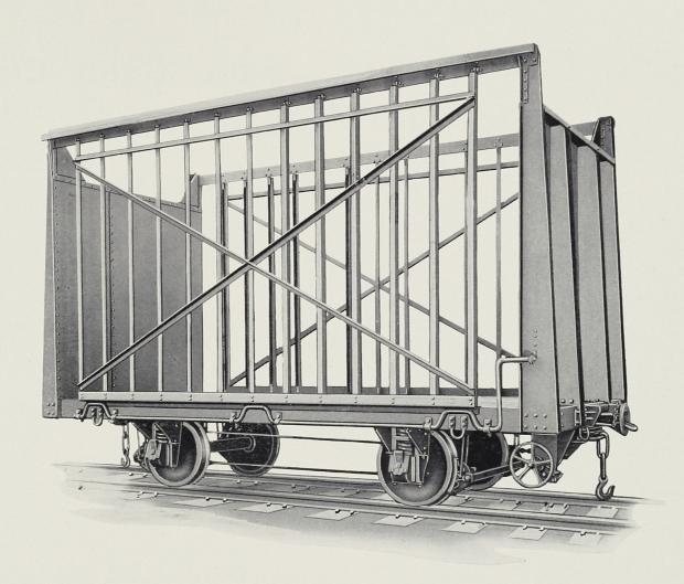
10-Ton Four-Wheeled Sugar Cane Car Built for Trinidad
