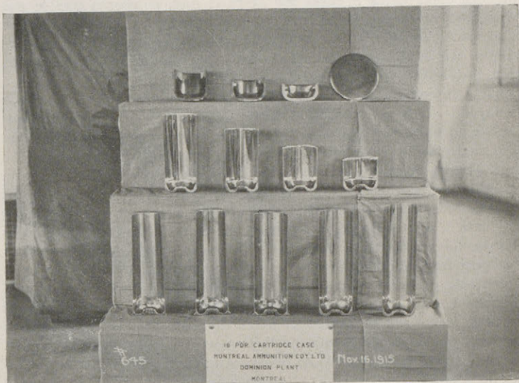
Fig. 24. Operations in the Manufacture of Cartridge Case.
