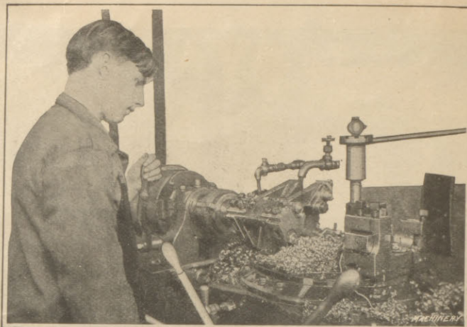
Fig. 21. First Rough-turning Operation on Shrapnel Shell in a Flat Turret Lathe
