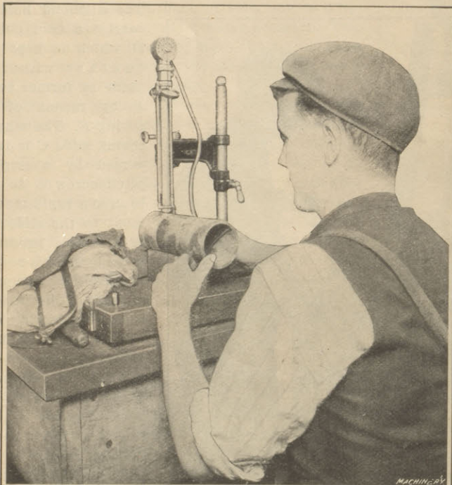
Fig. 25. Testing Hardness of Shrapnel Shells with Shore Scleroscope
