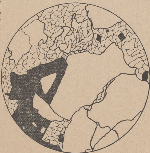
FIGURE I. Section of the granite showing cataclastic structure with deposition of secondary pyrite. Magnified 32 diameters.
