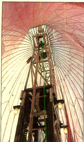
Diamond drill operating under cover at Hay West (see photo below)
