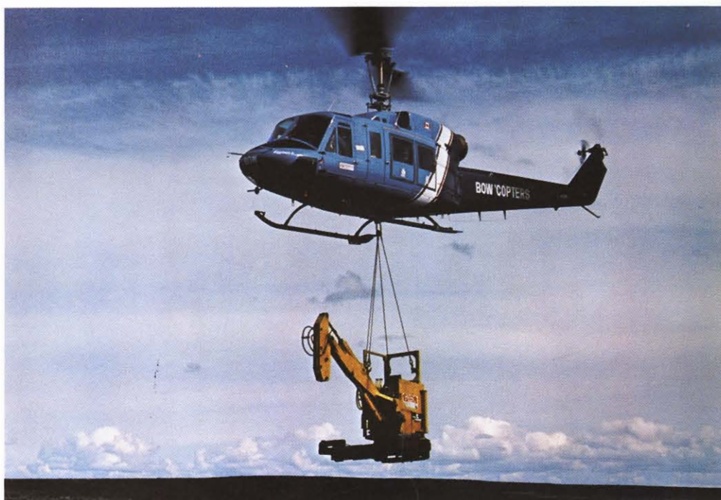
The 16-passenger Model 214B "BigLifter," shown carrying an oilfield pumping unit, is Bell Helicopter Textron's most powerful single turbine aircraft, providing more lift and speed than any Bell utility helicopter ever manufactured. It can lift payloads of up to 7,000 pounds, including pipe sections, utility towers and construction materials such as concrete and steel girders and beams. The ship has a top speed of 160 miles per hour.
