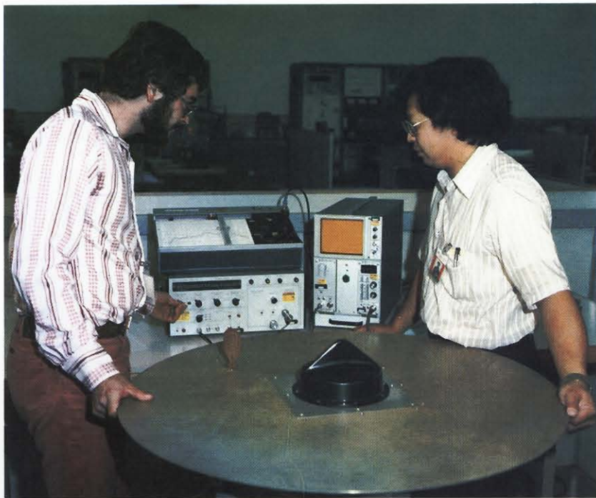
Radiation patterns of a Dalmo Victor "Compass Sail" direction-finder antenna are taken on a movable ground plane by engineers at Dalmo Victor's Final Test Facility in Belmont, California. Compass Sail is one of the newer electronic countermeasure systems that the Dalmo Victor Operations of Bell Aerospace Textron is producing for the U.S. Air Force, for use on first-line combat aircraft such as the F-16, the F-4 and the A-10.
