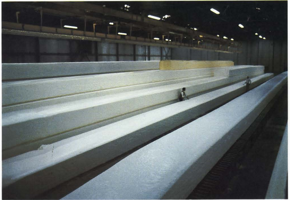
Buns of urethane foam 200 feet long are moved by conveyor into a curing area and stacked for storage by an overhead lift at Burkart Randall's Cairo, Illinois plant. The buns, produced by computer-controlled machines, are cut into hundreds of sizes and shapes for use as cushioning in automobiles and furniture.
