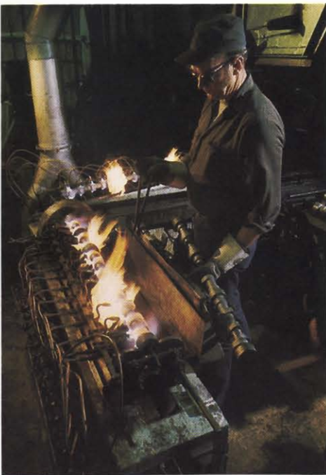
Camshafts made at CWC Castings are heat treated in a special flame metal hardening process that controls chemical and physical properties. The result is a tough product with excellent wear characteristics. In 1978 CWC will cast camshafts for a number of General Motors Divisions, for American Motors, and for Volvo of Sweden.
