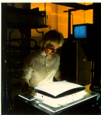
Left: Faceplates for color picture tubes are inspected for blemishes at the RCA Video Component and Display Division facility in Marion, Ind.
