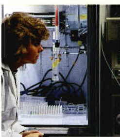
Refrigerated chromatographic columns are used to isolate and purify hormone receptors. Such techniques aid in discovering drugs to block receptors in the treatment of cardiac hypertrophy and hypertension.
