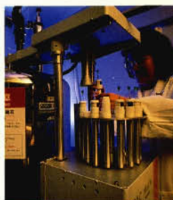
Chemists determine the molecular structures of new drugs using an NMR (nuclear magnetic resonance) device.
