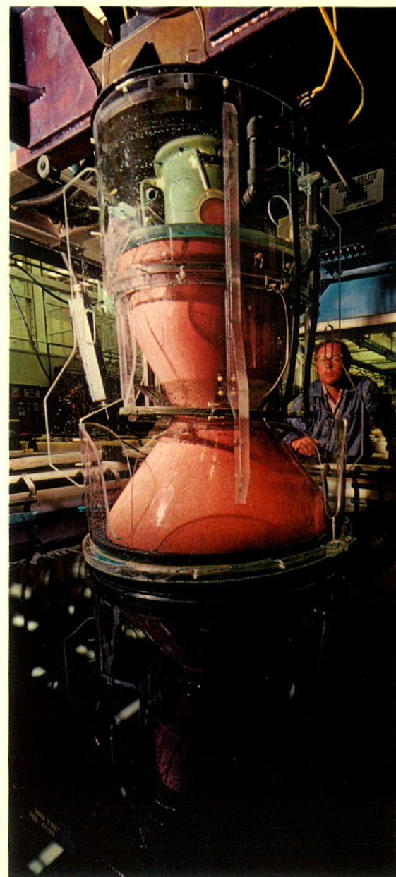
Rocketdyne uses a unique electroplating facility in the production of an advanced design combustion chamber for the Space Shuttle Main Engine.
