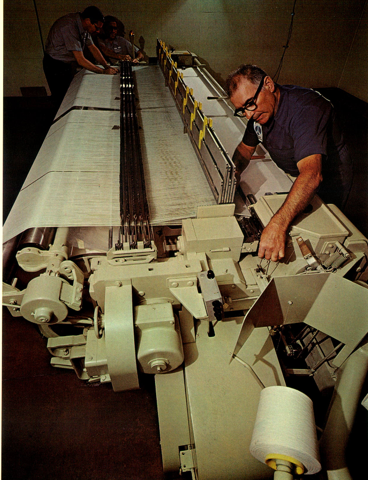
Designed to produce extra-wide cloth, the new Draper DML > loom weaves fabrics from 90 to 220 inches in width.
