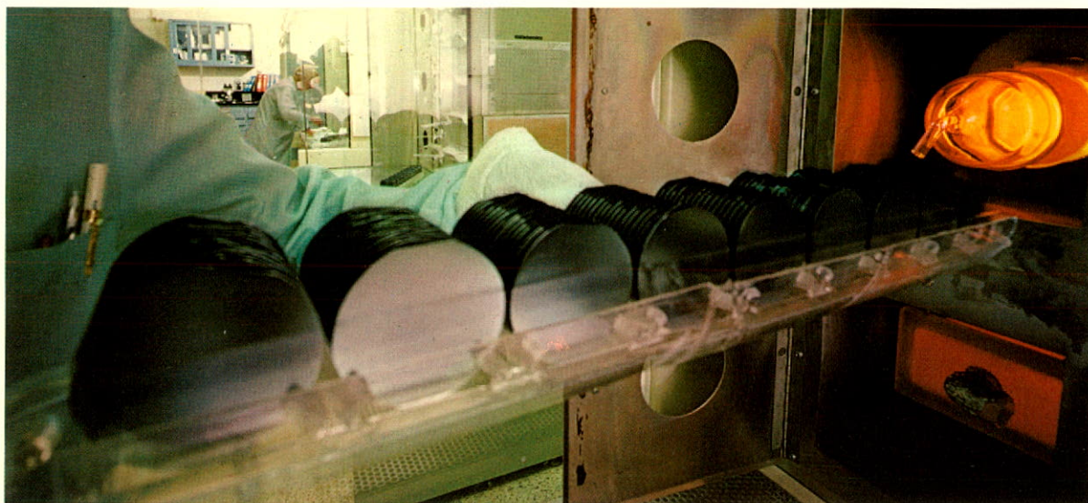
Wafers, containing as many as 100 electronic circuits each, are heat treated at temperatures up to 1000° C.
