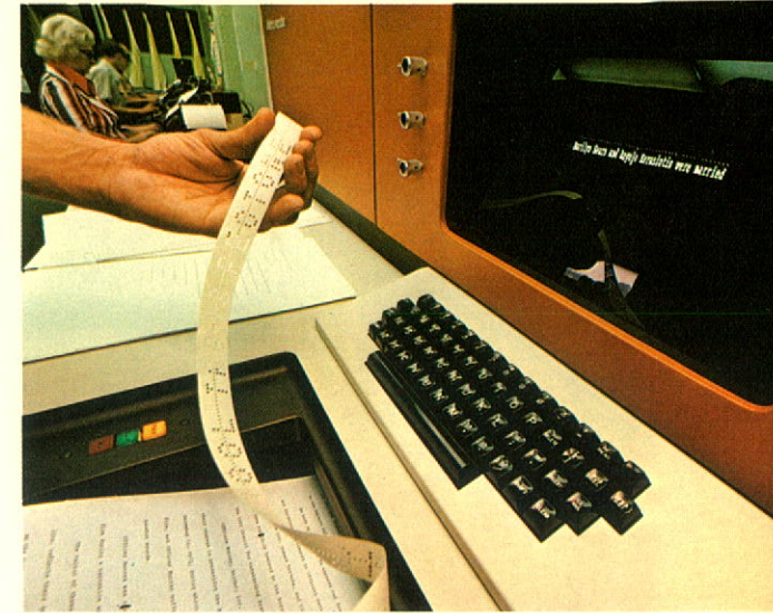
MGD's laser-equipped Metro-reader, an optical character reading machine, has been installed by some of the nation's leading newspapers.
