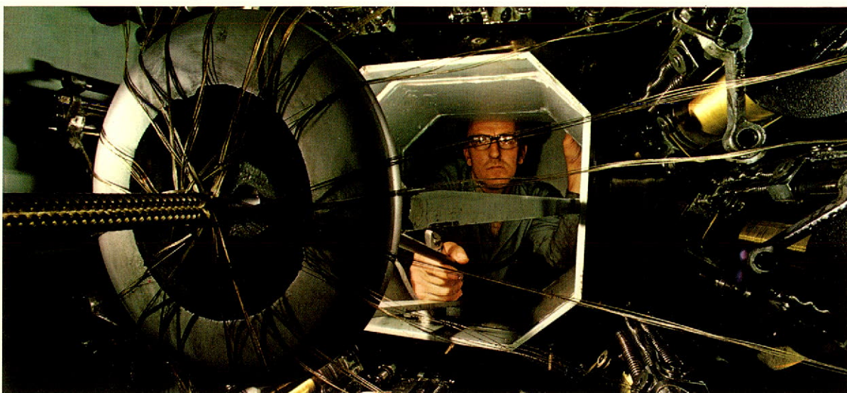
The new Rockwell 225-II braider, made by the Textile Machinery Divisions, is used by plants worldwide in the manufacture of reinforced hydraulic hose.
