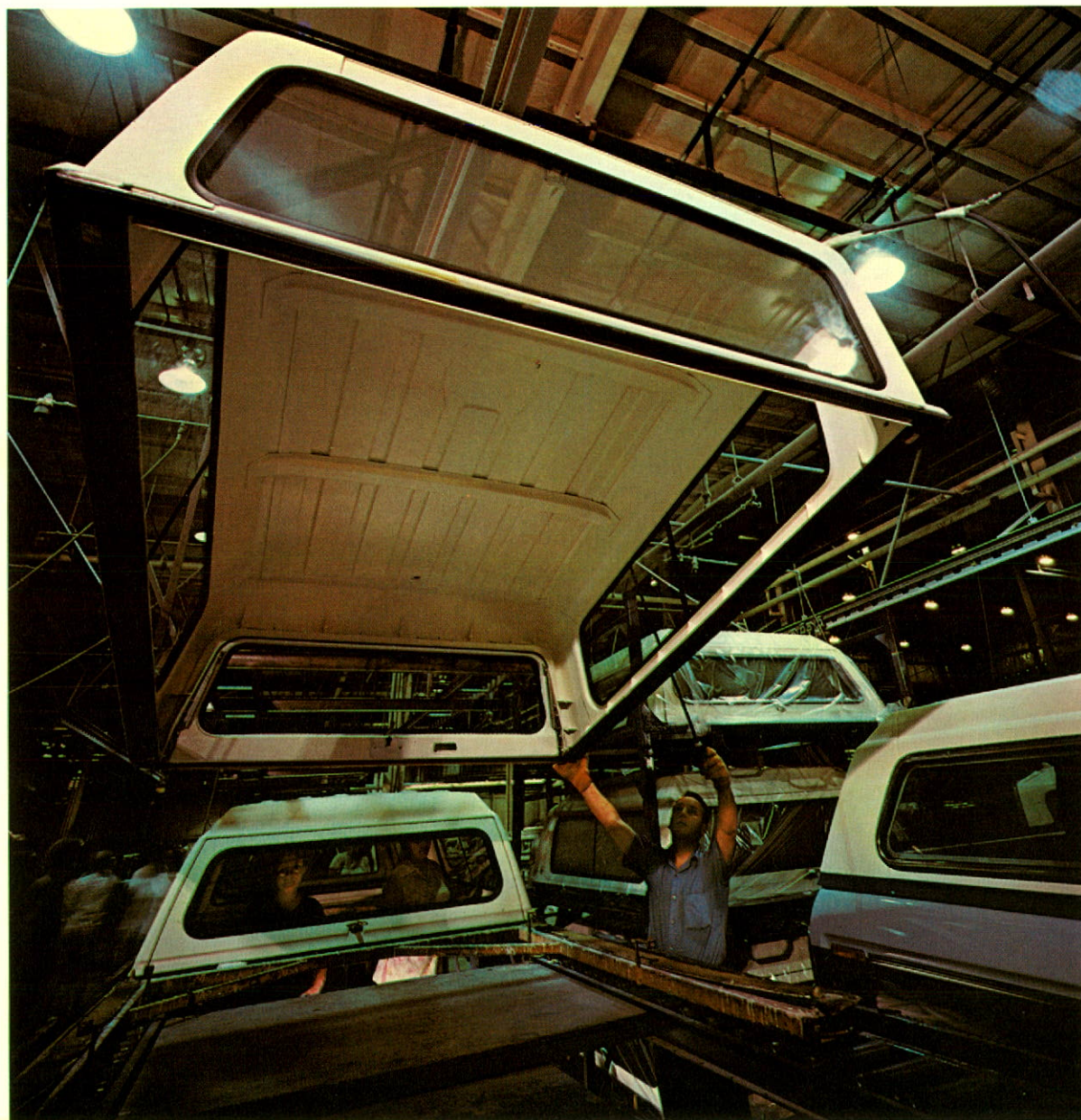
Fiber glass box covers for pickup trucks are produced at the Centralia, Illinois, plastics plant.
