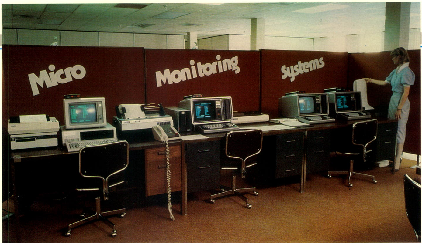
Micro Monitoring control room at Toronto. Computer print out provides hard copy of all monitored data when required.
