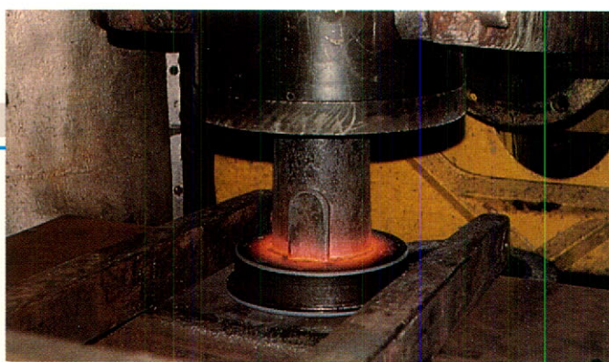
Die forging oil well connectors on 3,000 ton press.
