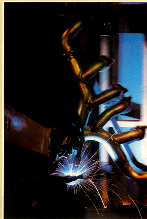
Robotic systems have virtually eliminated weld quality problems.
