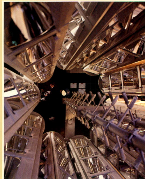
Computerized equipment measures the reflectivity of automotive headlamps.
