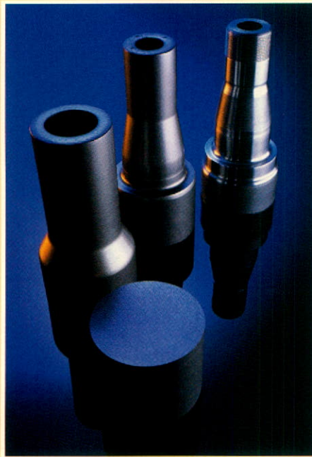
Through a series of progressive operations, a metal slug is shaped to near-final dimensions.
