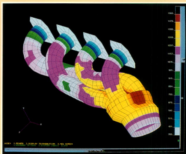
Workpiece characteristics can be evaluated by computers even before a part is manufactured.
