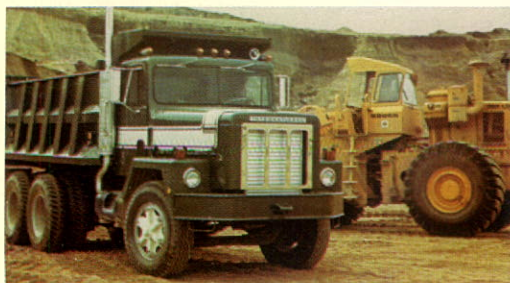
Trucks like this Series 5000 made by International Harvester Company of Chicago, Illinois, are sold in many parts of the world for use on construction projects for hauling fill, rock, gravel, sand or asphalt over long distances.
