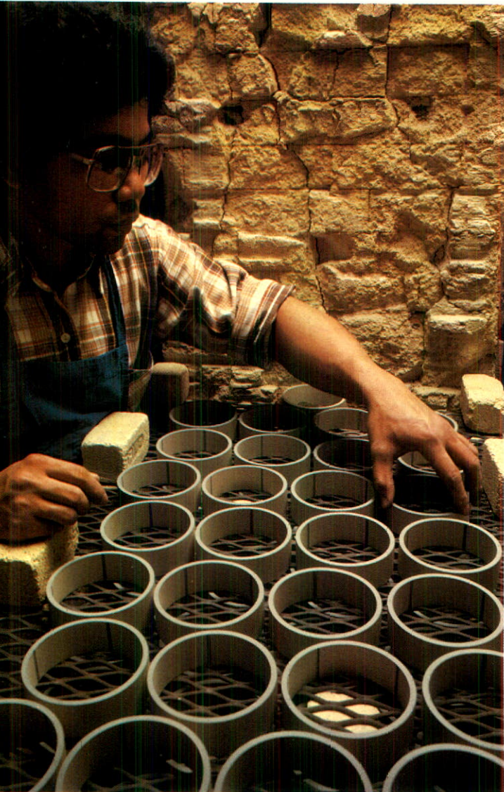
Kiln treating piezoelectric ceramic components
