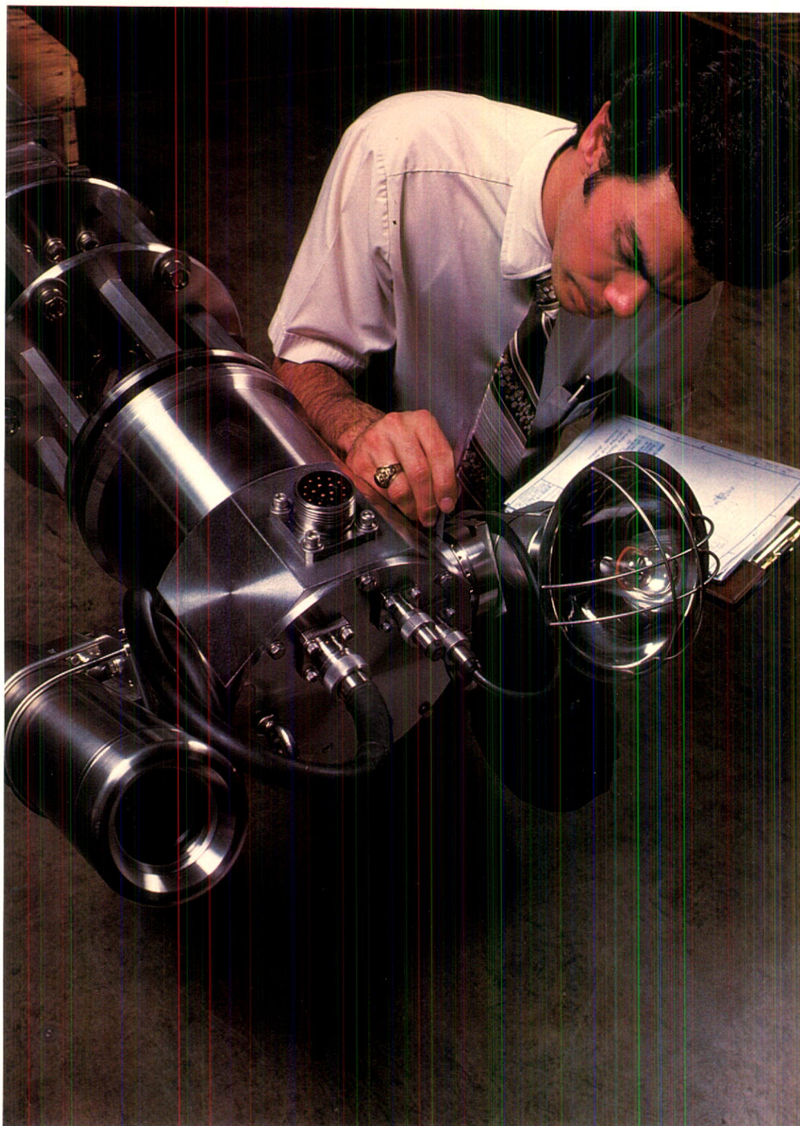
TV monitoring system for subsea drilling operations
