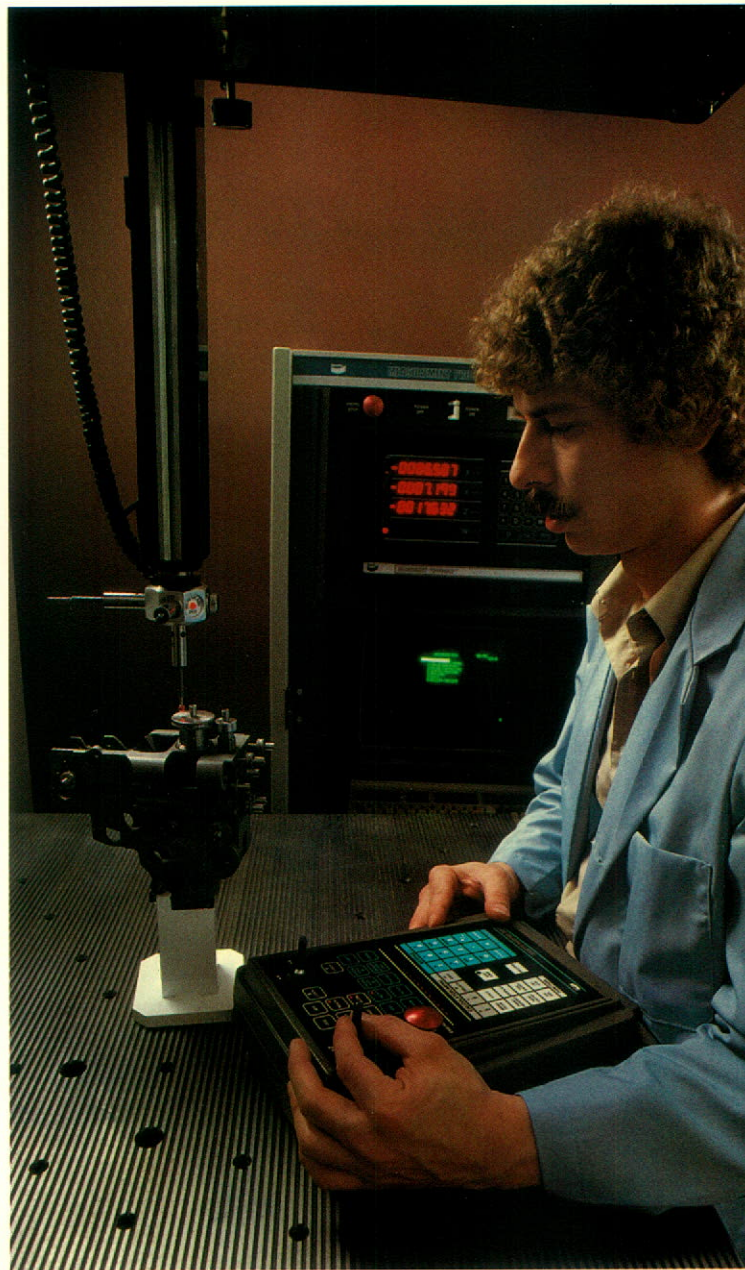
Direct computer controlled, coordinate measurement system
