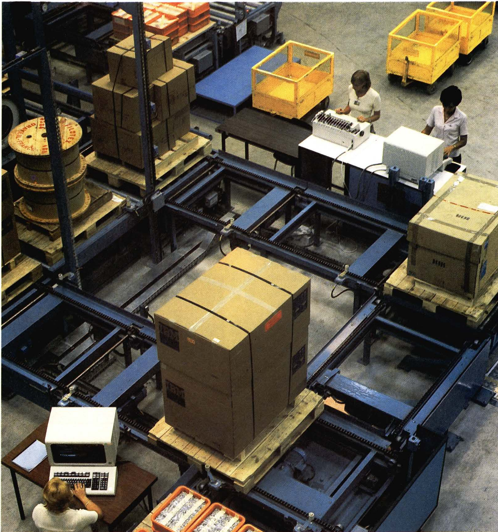
New computer-controlled materials distribution center at IBM France's Montpellier plant reduces costs and improves the handling and transportation of materials, as well as speeding the availability of parts to production lines for computers and data communications products.
