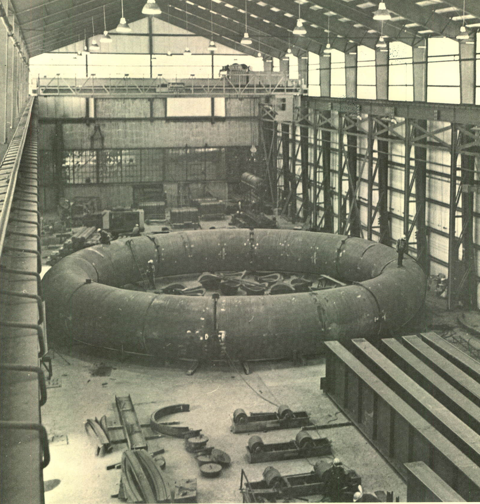
Fabricated and trial-assembled by the Plate Fabrication Division of TIW, this 60 foot diameter unit, approximately eight feet high, is one of the largest bustle pipes of its kind.
