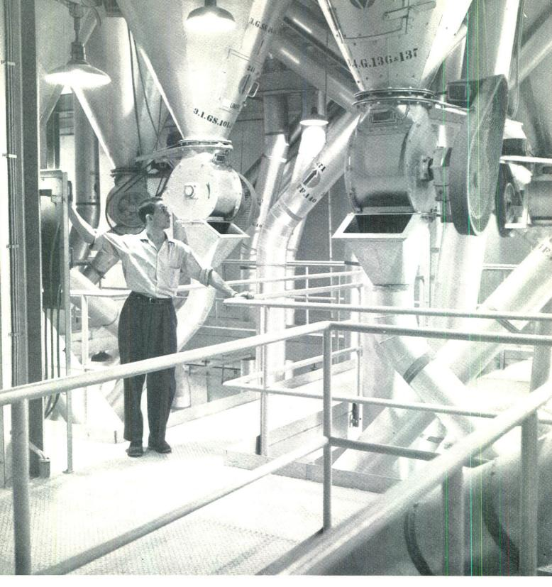
Clean, fluffy asbestos fibres pass through the bottoms of the cone-shaped cyclone separators shown at the new mill. Construction of the \$9.2 million mill, the world's newest and most modern, was begun two years ago. Now it is in full-scale operation and asbestos from this mill is being shipped to industrial consumers throughout the world.
