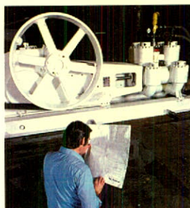
Mud pump (left) built by Koehring-Morgan Petroleum Equipment, moves manufactured "mud" that acts as medium to carry cuttings to top of hole in which an oil well is being drilled. Koehring-Morgan's entrance into oil field equipment market provides greater utilization of facilities in Ohio plant.
