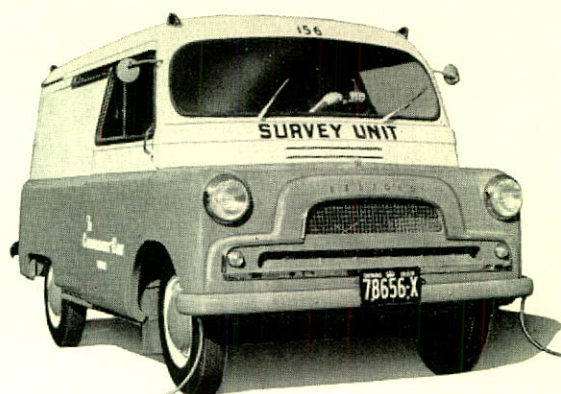
Infra-red mobile gas detection unit which provides a highly sensitive new method of surveying a distribution system rapidly and economically.
