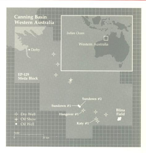
Since our 1981 Blina #1 oil discovery we have participated in the drilling of three successful appraisal wells, confirming the presence of the commercial Blina field. Production started in late September, 1983 at a rate of approximately 800 barrels of oil per day, making Blina the first producing field in the Canning Basin. The oil is transported by a newly-constructed pipeline from the Blina field to a loading terminal, then trucked to
