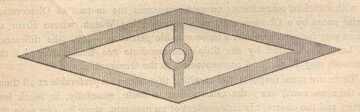
for the straight Needle; the Card is as before, with the addition of four talc Vanes fixed beneath and perpendicular to it, and at right angles to each other; these are designed to check the Vibrations, and to cause the Needle to settle more speedily, by reason of the resistance which they experience from the air in the Compass-Box; the Needle, Card, and Vanes, with the Agate Cup and Screws, weigh altogether 1731 grains.
