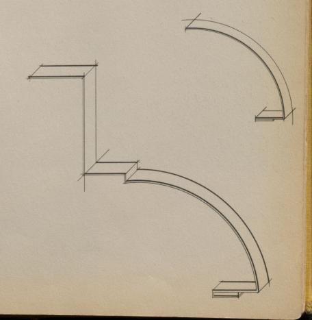
Sketch of a cantilever system for a display fixture. Bent metal.
