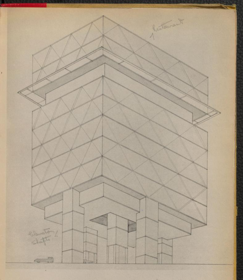
Department Store. Elevated Building. Floor free for circulation. Five elevator shafts, the central shaft leading into an open gallery. Each elevator shaft surrounded by show windows. On the tenth floor is an open-air restaurant.
