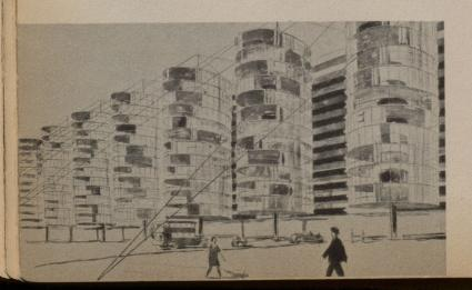
Series of suspended houses. "The mast is secured against wind-pressure snapping and every load which results from the suspended stores. The spherical end of the mast which stands in the ground is 32.5 cm. in diameter and is made of steel. It lies in a corresponding steel socket, which is secured in a round concrete foundation 9.5 m. in diameter." "The masts are spanned by well isolated
