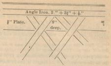
Allow 100 cwts. per square inch of net section in tension, 65 cwts. per sq. in. of gross section in compression, and a shearing stress on the rivets of 100 cwts. per sq. in.
