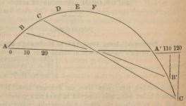
ordinates from the line BB1 will give the bending moments along the girder (the distance along the girder being measured horizontally from
