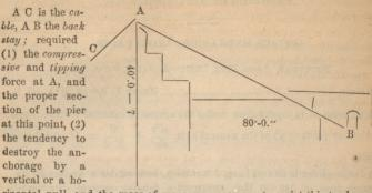
rizontal pull, and the mass of masonry necessary to resist this tendency.
