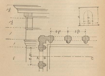
A. Above is sketch plan of angle of courtyard, treated as a one storey open arcade with engaged columns of the Roman Doric Order, which are 8 feet from centre to centre. Upon this is to be added a second storey, forming an open gallery or arcade, after the fashion of an Italian loggia. This, while necessarily classical or renaissance in character, is left free to candidates to design in detail.
