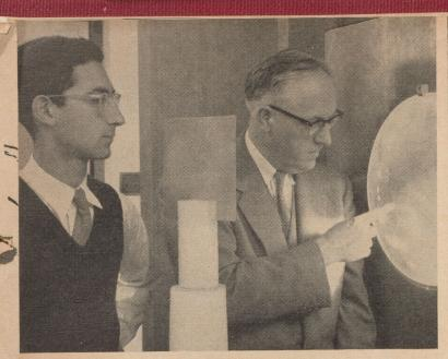
Prof. Woonton, Laboratory Director, explains to student Issie Shkarofsky, Montreal, the passage of microwaves through a solid plastic lens and the measurement of those reflected back to the source by a metal plate.
