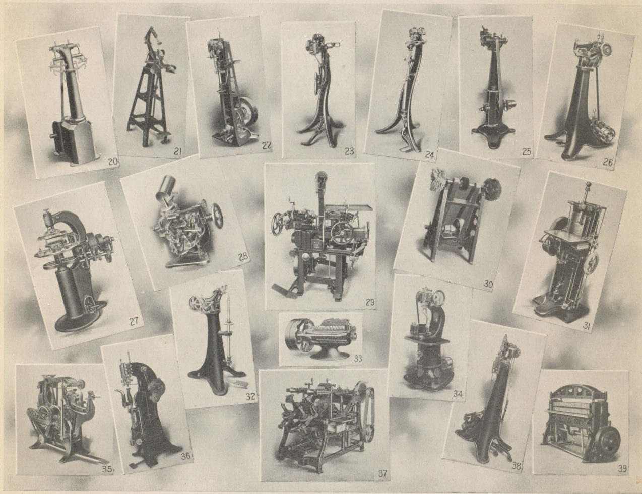
20. Union Twin Edge Setting Machine—Model S 21. Goodyear Heel Turning Machine 22. Imperial Heel Breasting Machine—Model B 23. Universal Double Clinch Machine 24. Goodyear Welt Indenting and Burnishing Machine 25. Feather Edge and Shank Reducing Mch.—Model H 26. Goodyear Universal Welt Beating Machine
