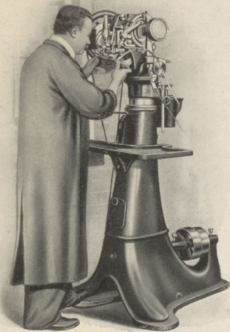
GOODYEAR WELT SEWER WHICH SEWS SHOE UPPER TO INSOLE AND WELT, LEAVING SHOE PERFECTLY SMOOTH INSIDE
