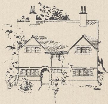
ELEVATION FOR A VILLA, FT. FRONTAGE, TO BE BUILT IN STONE AND CONCRETE OR BRICK.
