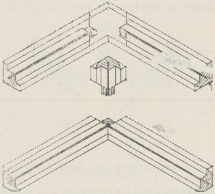
COUNTER CASES: JOINTS BETWEEN TOP FRONT CORNER OF RIM AND CORNER POST.
