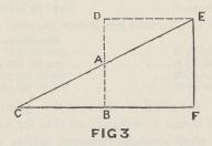
E C F represent one-half of a roof. The weight upon the slope, C E, may be considered as concentrated at A, midway between the ridge and the foot of the rafter. Draw D B, parallel and equal to E F, and if D B represents the weight and stress upon C E then C B will represent the horizontal thrust against C. At quarter pitch, D B is equal to C B, so that the thrust is equal to the load.
