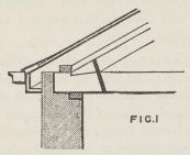
shown in section at fig. 1. True there is a greater length of common rafter and a greater extent of roof covering than in the parapet roof, as shown at fig. 2; but then, in addition to the advantages already enumerated, it will be seen that in fig. 1 the principal rafter
