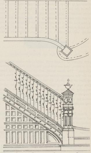
Fig. 1.—Plan and Elevation of Stairway and Railing.
