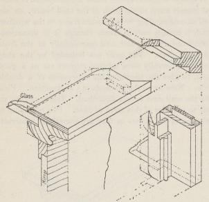
COUNTER CASES: JOINTS BETWEEN BACK AND END OF TOP AND BACK CORNER UPRIGHT, WITH SECTION OF FLAP.
