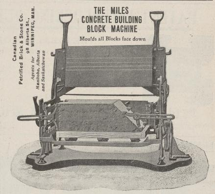
The Miles Machine makes Gable Blocks face down in any design, without leaving a ragged edge.
