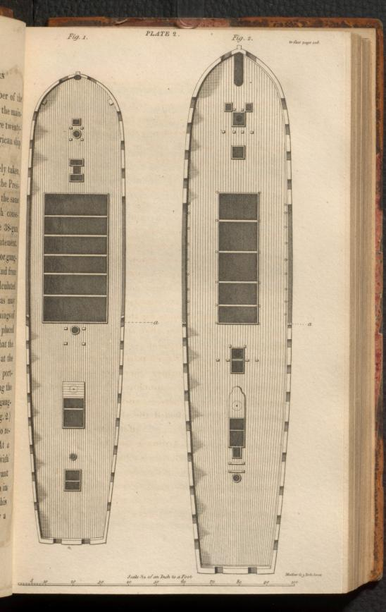
long gun) being intended to be shifted there, when necessary. The reason of the upper decks of the two ships differing so little in width, is, that fig. 1. is, what is called, wall-sided, while fig. 2.'s sides fall in as they rise. Upon the maindecks, the due breadth of each ship is preserved.
