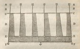
**BB**, the hawsers leading from the capstans to the nets. cc, the water's edge. DD, strong nets running from the beach into the sea: they reach from the bottom to the surface of the water. EE, large casks, used to buoy up the outer or great net, which runs parallel to the shore. FF, small anchors, confining the outer net close down to the ground. The hawsers from the capstans being slackened, the smaller nets DD sink to
