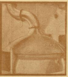
Sufficient hops and malt to produce thousands of gallons of ale are boiled together at one time in the immense Brew Kettles of Dawes Brewery,
