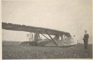
The Falcon intermediate sailplane, an advanced type of glider suitable for soaring and sailplaning.
