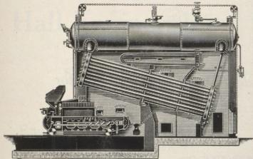
Babcock & Wilcox Patent Water Tube Steam Boiler, Superheater and Mechanical Stoker.
