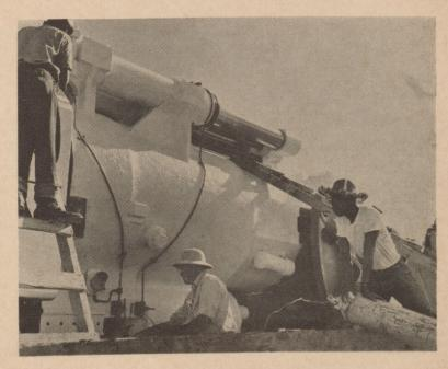
Ben Tubman, gun expert, centre, works patiently building up pressure in faulty recoil cylinder atop 16-inch gun.
