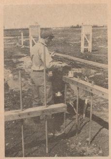
Measuring soil movements and soil temperatures
