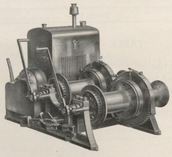
Rope pull 2,500 lbs. at 150 ft. a minute. A'dependable machine made with cut gears, asbestos lined frictions and brakes, machined and bronze bushed drums and operated by a four-cylinder Le Roi heavy duty engine.
