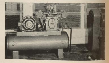
... for pumping tires, paint-spraying, engine-starting, operating instruments and controls or other purposes requiring small volumes of air at a wide range of pressures.
