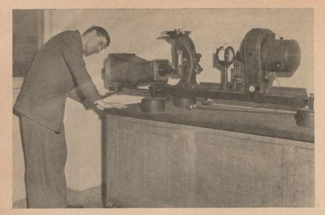
THIS INSTRUMENT in the department of metallurgy is virtually priceless as there are so few of its kind left in existence. It is a Zeiss metallograph used for microscopic study of metals and alloys. Magnification as high as 2,000 times may be obtained. Dr. J. P. Ogilvie, B.Eng. '43, is shown here using the instrument.
