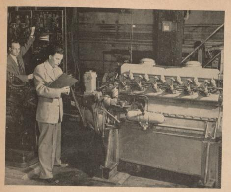
PART OF THE VALUABLE CONTRIBUTION to industry in the department of mechanical engineering is to test the power of diesels. Here J. C. Cherna, left, and W. Bruce, both on the staff, are checking the power output, fuel consumption and efficiency of a diesel.
