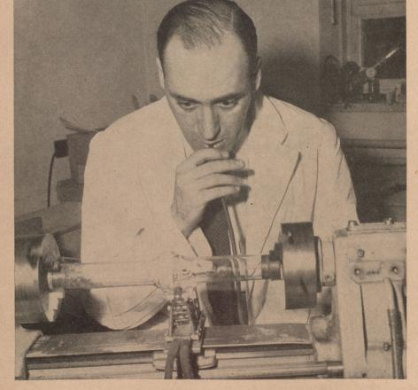
AN ANCIENT CRAFT is seen here in a modern setting. Dr. Sydney Wagner, Ph.D. '51 is using a glass lathe in the electronics laboratory to fashion one of the test tubes used in the research work carried on there.
