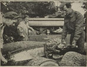
Mobile Pneumatic Power for Mobile Forces. Top: A "Utility" Pneumatic Hoist operating a drag scraper. Centre: The portable compressor unit can travel at high speed and may be quickly placed in service. Bottom: Pneumatic Saws and Woodborers speed logging and timber assembly operations.
