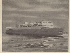
This powerful, diesel-electric, ice-breaking train ferry keeps communications open between New Brunswick and Prince Edward Island. All the electric propulsion equipment was designed and manufactured by Canadian General Electric.
