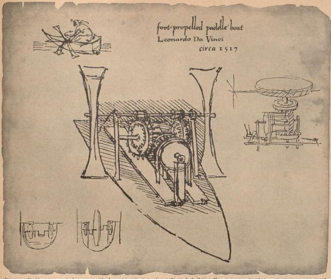
LEONARDO DA VINCI possessed what was possibly the most imaginative and versatile mind of all time. He was, among other things, an artist, an engineer, and an inventor. Reproduced here are original sketches by Da Vinci for a foot-propelled paddle boat, showing details of gear mechanism, paddles, cam, and fly wheel.
