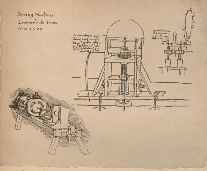
LEONARDO DA VINCI, in addition to being an artist, engineer, and inventor, was also a superb craftsman. Reproduced here are original sketches by Da Vinci of boring machines—one for boring cylinders, the other featuring a unique self-centering device.
